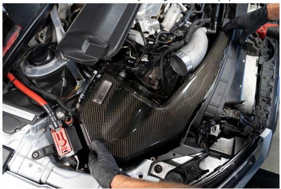
Reinstall radiator allen bolts, Silicone elbow and hose clamps, radiator cover and hood latch, then the engine vanity cover.
