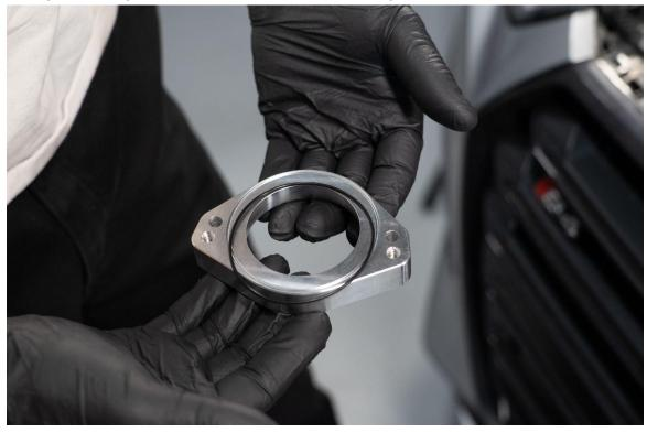
Install compressor housing adapter to turbo using two supplied 5mm flat head screws taking note of the orientation of the adapter.
