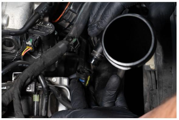
Install supplied O-Rings into the grooves of the Compressor housing adapter. A tiny dot of superglue in the groove can help hold it in place during installation.
