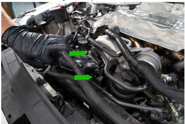
Remove the lower breather hose by pushing in both sides of the release tab and pulling down. You can now remove the factory turbo inlet from the vehicle.
