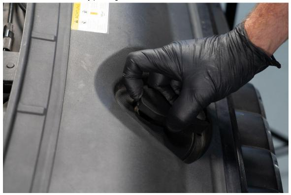
Remove plastic radiator cover by pulling up on the front edge, then pulling straight towards the front of the vehicle.
