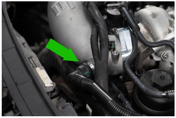
Reinstall Carbon intake. Space is tighter with the upgraded inlet. We recommend putting some painters tape on the inlet to help minimize the chance of scratching the airbox. To fit the carbon box without scratching it, first turn the intake roughly 90 degrees towards you, then insert the pointed end of the intake into place.
