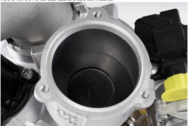
Reinstall the OEM Turbo Muffler O-Ring in the groove on the top edge of the Canister.
