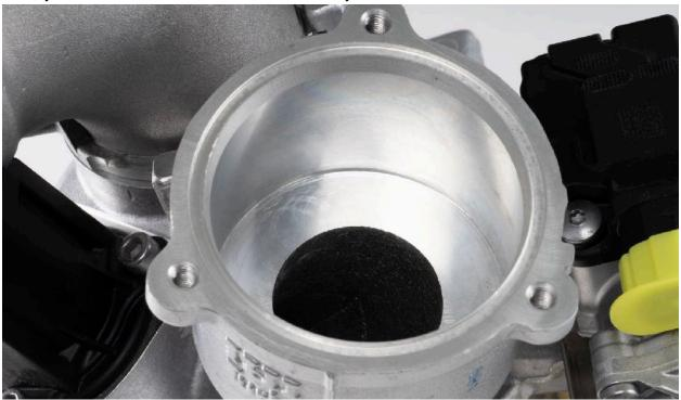
Insert the Perfect-Seal Gasket into the Turbo outlet so that it sits flush at the bottom, inside the Turbo Outlet Canister.
