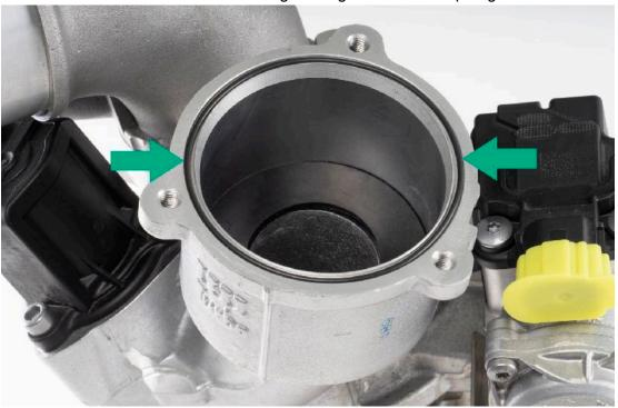
Insert the IE Turbo Muffler Delete into the canister with the logo facing outward and install the three 5mm Allen bolts.
