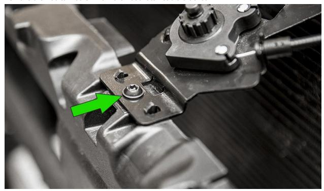
Push the two securing tabs forward and pull up to remove the hood release cable bracket.
