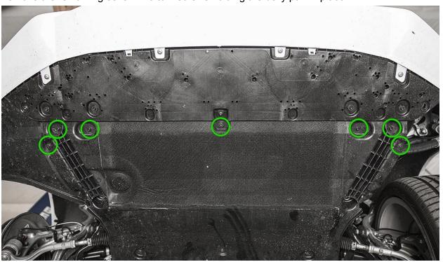
Remove belly pan from vehicle by sliding backwards.
