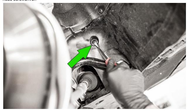
Remove the three plastic nuts with a 10mm socket and the eight T25 torx screws in the wheel well that secure the wheel liner.
