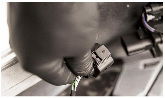
Verify all harness connectors are disconnected and free, then completely remove the front bumper.
