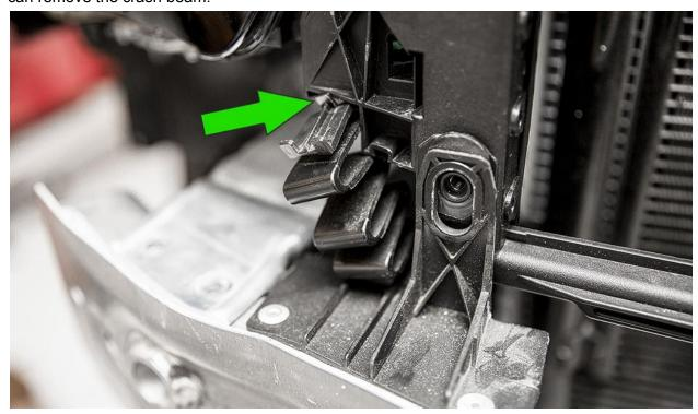
Remove the two upper T30 torx screws from the plastic support bracket.
