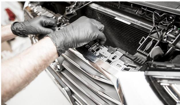
Release the bumper cover from the fender by pulling on the outer top edge. Repeat on both sides. *Note: Use caution during this step to not break the plastic clips that fasten the bumper.*
