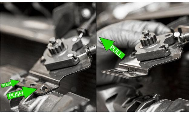
Disconnect the two hood release cables from the bracket.
