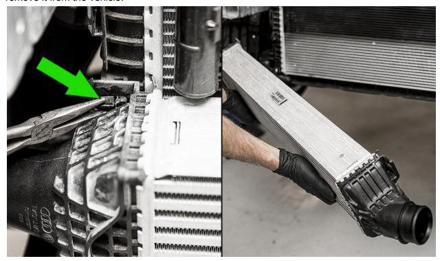
Using the 4 supplied allen bolts and 5mm allen wrench, install the upper support brackets to the IE FDS intercooler end tanks as seen below.
