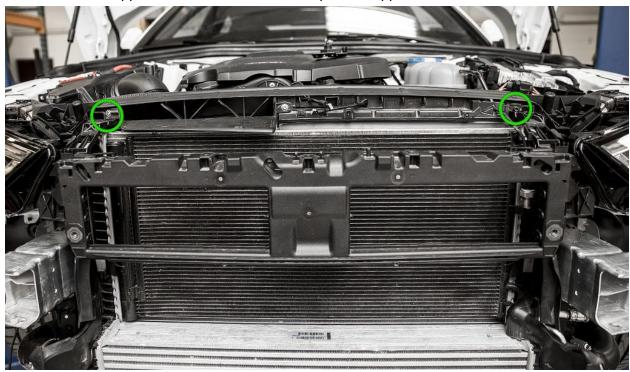
Using a long T30 torx driver, remove the remaining two T30 torx screws located in the center of the plastic support brackets on both sides, then fully remove the bracket assembly.
