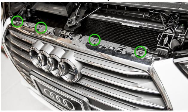
Release the grill from the bumper support bracket by gently pulling the clips up and forward.
