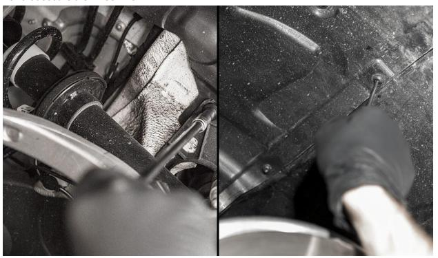
You can now fully remove the lower wheel liners. Repeat this process on both sides.
