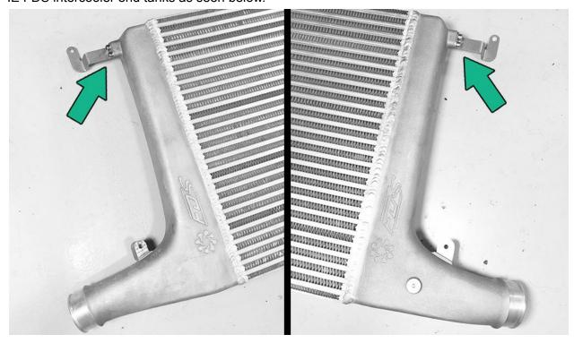
Using the 4 supplied allen bolts and 5mm allen wrench, install the lower support brackets to the IE FDS intercooler end tanks as seen below.
