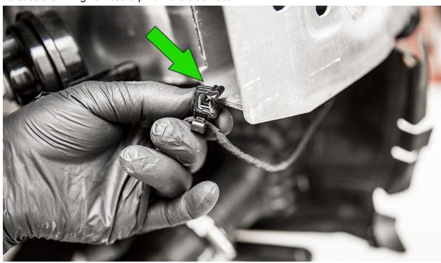
Unclip any harness connectors located on the crash beam and set out of the way.
