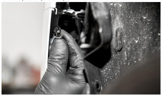
Using a long extension, locate and remove the T30 bumper to fender bolt, one on each side.
