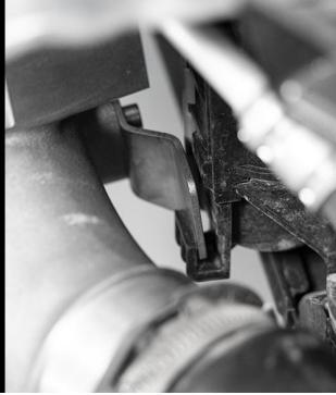
Insert the bracket spacers (2) and supplied screw bolts (2) to fully secure the intercooler top brackets to the vehicle with a T25 torx driver.
