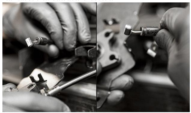
Release the wiring harness clip from the crash beam.
