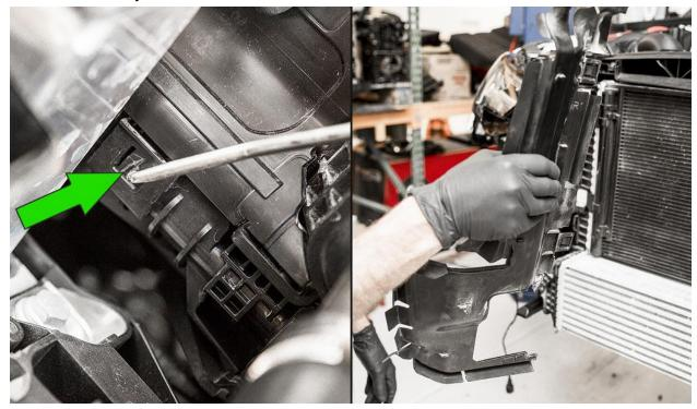
Loosen the stock hose clamps from the intercooler hose, then pull back to remove it from the OE intercooler. Repeat on both sides.
