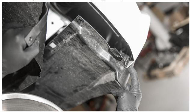
Remove the plastic bumper to fender push-lockers, one is located on each side.
