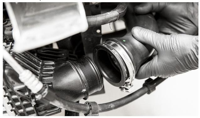
Using a pair of needle nose pliers, release the two pinch clips from the stock intercooler and remove it from the vehicle.
