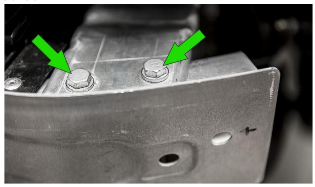
Remove the two T30 torx screws securing the crash beam to the plastic support bracket on both sides.
