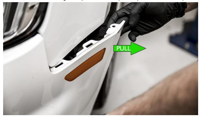
Pull the driver's side of the bumper cover forward and disconnect all electrical connectors located inside. *Note: Do not pull bumper too far forward in this step, it can damage the bumper harness.*
