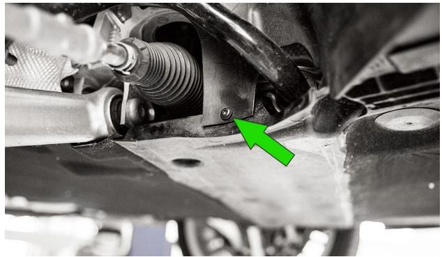
Remove the remaining seven T25 torx screws holding the belly pan in place.
