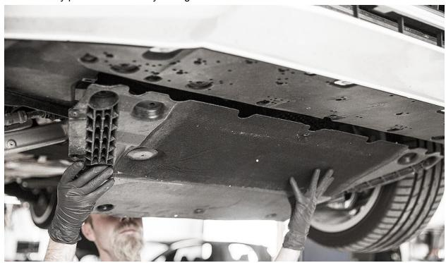
Remove the four T30 torx screws and one T25 torx screw from the underside of the bumper that secures it to the radiator support.
