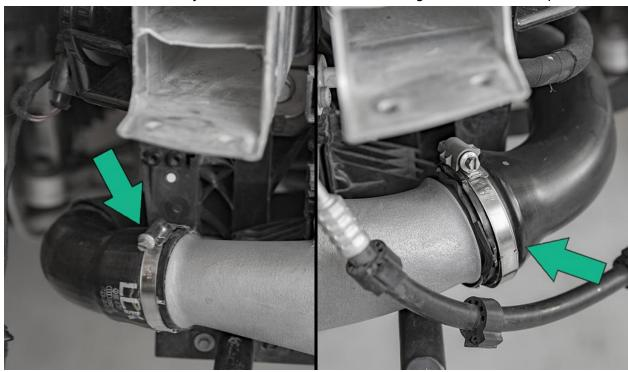
Install either a water methanol nozzle or the included plug with a 3/16" allen and thread sealant. begin reassembling the car by following the reverse of the procedure detailed above.
