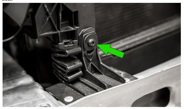
Release the two plastic spring clips by pushing down on the tab and pulling forward. Now you can remove the crash beam.
