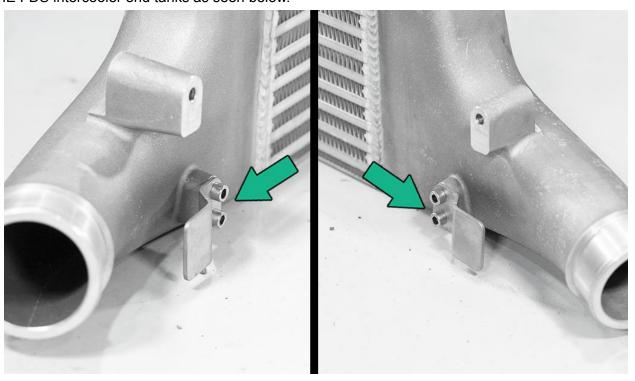
Align the intercooler onto the vehicle and support it in place. *Note: a second set of hands may help here*.
