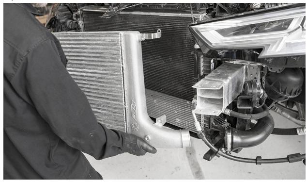
Align and seat the lower brackets into the factory radiator slots.
