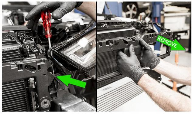
Remove the plastic air shrouds by pushing in on the two retainer tabs (one top, one bottom) and pulling forward. Repeat on both sides. Be careful to not damage the shrouds as you will need to re-install them on your new intercooler.
