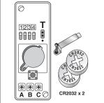
Remove the locking screw from the battery fastener. Insert 2 x 3 volt CR2032 Lithium batteries (Byron SX-100) in the battery compartment, ensuring the battery polarity matches the internal markings, then tighten the screw on the battery fastener to hold the batteries firm in it's compartment.
