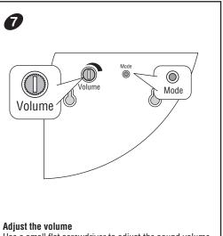
Use a small flat screwdriver to adjust the sound volume Mode Selector
