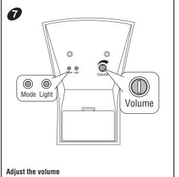
Use a small flat screwdriver to adjust the sound volume Mode Selector
