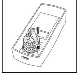
Remove the locking screw from the battery fastener. Insert 2 x 3 volt CR2032 Lithium batteries (Byron SX100) in the battery compartment, ensuring the battery polarity matches the internal markings, then tighten the screw on the battery fastener to hold the batteries firm in it's compartment.
