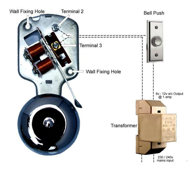
The Imperial London Striker bell / buzzer is powered by a transformer only, with an output voltage requirement between 8 and 12 v a/c, and power output of 1 amp. If 2 bells are wired into the same system then a transformer with a 2 amp output is required.
