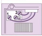
Type V/A On-period Terminals LTW 3811 8V WS AC 8V/0,7A Short time 20s 1,2 LTW 3811 24V WS AC 24/0,23A Short time 20s 1,2 LTW 3811 230V WS AC 230V/0,05A Short time 20s 1/L,2/N,⊕ LTW 911 8V WS AC 8V/0,7A Short time 20s 1,2 LTW 911 24V WS AC 24V/0,23A Short time 20s 1,2 LTW 911 230V WS AC 230V/0,05A Short time 20s 1/L,2/N,⊕
