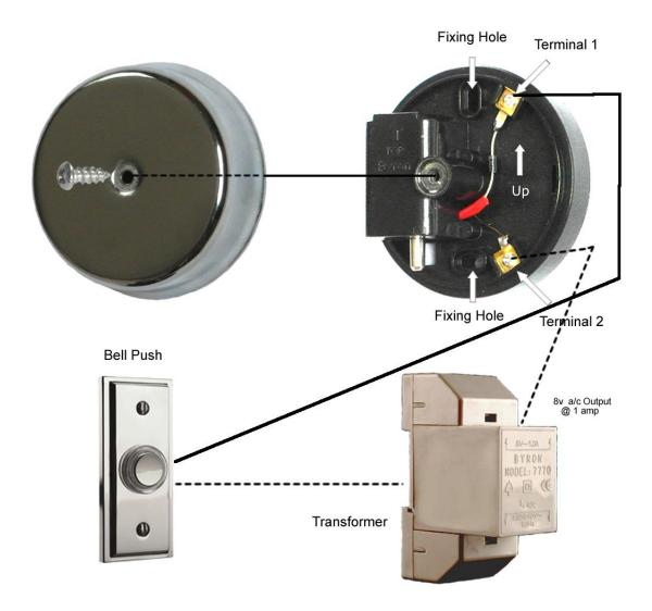
The bell system is wired in a series arrangement with the underdome bell, bell push button and transformer all part of the circuit. When the bell push is pressed, this completes the circuit, power passes through the bell and the bell continues to ring as long as the bell push is pressed.
