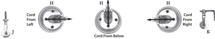
NB Use minimum Cord length and number of Pulleys so as to facilitate optimum Inner Spring tension.
