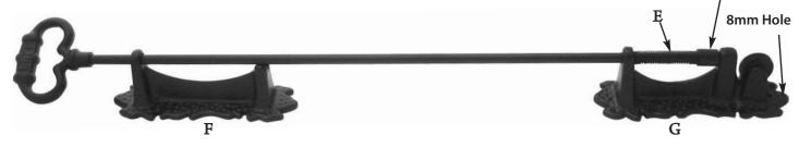
**3.)** Locate the Bell Pull assembly in a suitable position on the outside wall so that, when an 8mm hole is drilled to take the Cord from over the Black Pulley, the hole will avoid any objects placed on the inside wall of the house. Mark and drill 4 screw holes 6mm each in the Top and Bottom Mounting Brackets ensuring these are fixed and lined up with the previously drilled 8mm hole at the top.
