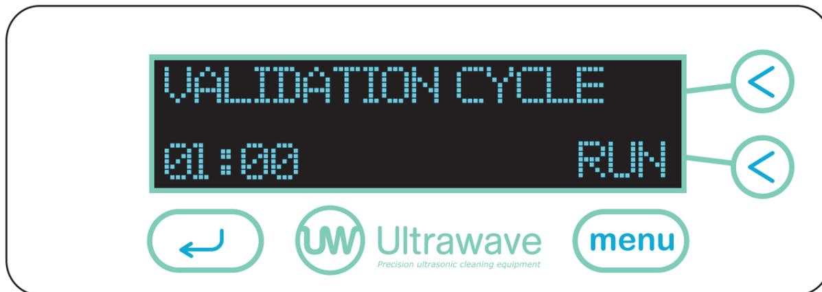
To run a validation cycle press RUN, the ultrasonics will operate for 60 seconds and a countdown will be displayed to indicate the remaining time.
