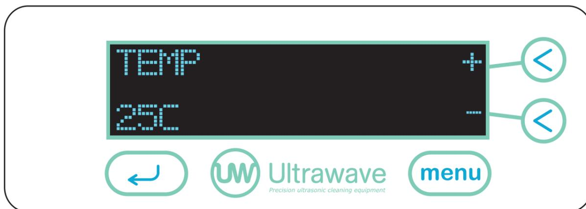
During normal operation, ultrasonic energy will heat the cleaning liquid by up to 15°C per hour. Your hygea d3ntal cannot cool the cleaning liquid. If the liquid temperature becomes too hot, you must either let it cool down or refill the bath with cooler water.
