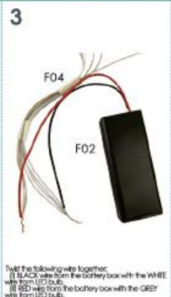
Wrap the bare wires with adhesive tape F04. Make sure the LED lights are on.
