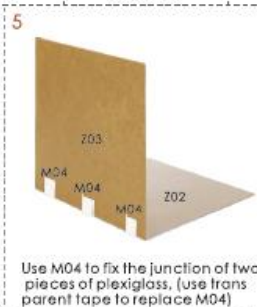
scale:1:11 Z02 plexiglass (transparent) 26*20*0.18cm (1 piece)
