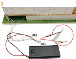
Put all gray wires with battery boxed wires together, and put all white wires with battery box black wire together. Wrap the bare wires with adhesive tape J03. Make sure the LED lights are on.
