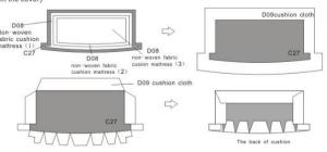
Paste another B27 wood onto the back's middle of the clipped cushion, then put cloth of the clipped D09 cushion, paste and fold a piece of cloth with a width of 0.8 cm according to the dotted line, then paste around the leading edge of the cushion.
