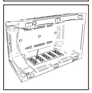
Place the window grate on the interior of the kennel. Align the grate with the window openings. Mark the mounting holes.
