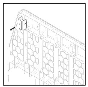
Remove the screw, and take off the security latch cover. Discard the latch cover.
