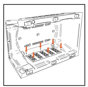
Insert supplied screws into designed points, and install grates using by twisting screws with applied manual force.
