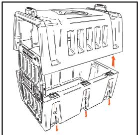
Using a 7/6" wrench or rachet, remove the screws and washers fastening the upper and lower halves of the kennel.
