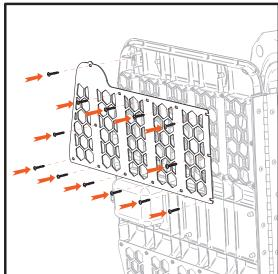
Place grate over windows and align the screw holes. Install the thirteen screws to secure the grate in place.
