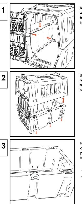
Remove three cap screws and washers that attach door frame to upper half of the kennel.
