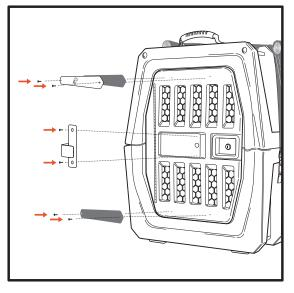
Next, use 2 screws to mount each magnetic plate. One to the top and one to the bottom of the door. With the 2 remaining screws, mount the retainer clip to the door at the nameplate location with the clip facing the paddle latch.
