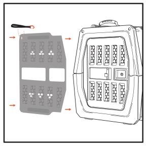
The magnets in the door cover are extremely strong, however, in the event of high winds, we want to ensure you do not lose your door cover. Using the provided security lanyard, feed loop through the grommet in the corner of the door cover. Thread the aluminum hook through the loop and pull tight. Attach the aluminum clip to the grate of the door to secure.
