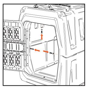
Reinstall the upper and lower halves of the kennel. Finally, reinstall three cap screws and washers in the door frame.
