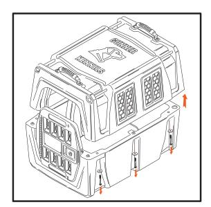
Using a 7/16" wrench or ratchet, remove the bolts and washers, fastening the upper and lower halves of the kennel.
