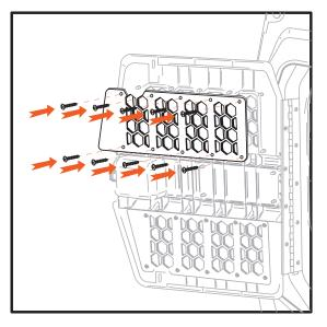
To install the Chew Kit on the door place grate over windows and align the screw holes. Install the ten screws to secure the grate in place.
