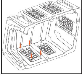
Line up the existing holes with the original kennel hardware.
