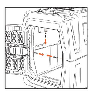
To install the Chew Kit on the windows use a 3/16" hex key to remove 3 cap screws.
