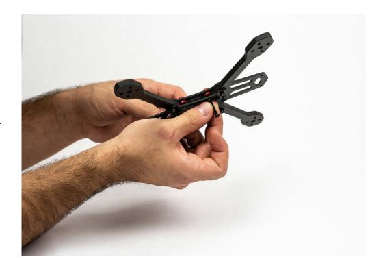
Insert the M3x20mm screws from the bottom, these will be used as your stack screws (4 in 1 ESC and Flight Controller)
