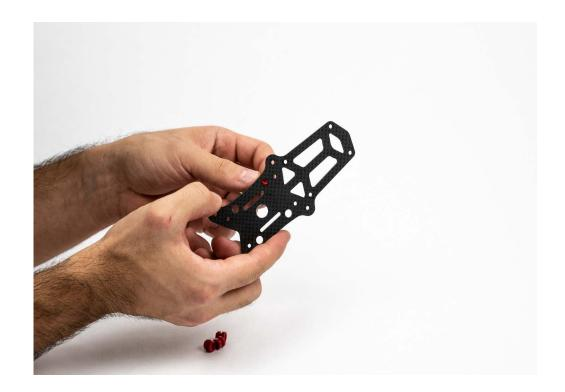
Insert all 4 flight control isolation grommets into the appropriate cut outs in one of the main plates.
