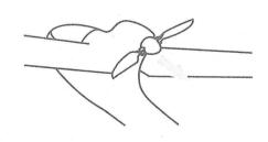
Remove the propelleras the direction of the arrow, then replaceaew one.
