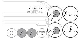
After bluetooth connected, short press "§1" or "§2" to easily switch between multiple devices.
