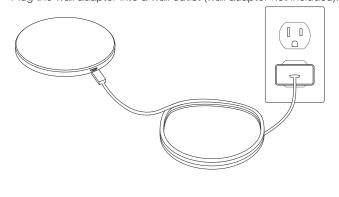
**Step 3:** Place your Qi-enabled device on top of the wireless charger. An LED light will power on to indicate the phone is charging.
