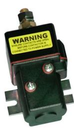
Supplied with 1x or 2x IP66 latching contactors—contactors are "bistable" which means they pull power only to transition between their on and off for maximum efficiency.
