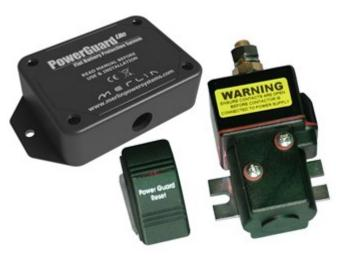
PowerGuard Lite provides basic flat battery protection. After voltage has reached a pre-set value for a pre-set time, the unit will disconnect batteries to prevent damage through excessive discharge and retain enough power to ensure engine re-starting. After activation, batteries are reconnected using a dash-mounted press switch.
