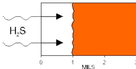
This testing is the same whatever the substrate that the Intercept is coated onto. The corrosion protection is directly tied to how much Intercept is available - how thick the coatings are. The thicker the coating, the longer the protection, on any substrate.
