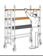
Fit two diagonal braces (blue) in opposing directions between the 1st and 3rd rungs. Ensure that the frames are vertical and level by checking with a spirit level and setting the adjustable legs as necessary. Fit stabilisers. Fit the next pair of end frames and check the frame interlock clips are engaged.
