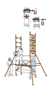
Fit two pairs of diagonal braces in opposing directions between the 3rd and 5th rungs and the 5th and 7th rungs Locate a trapdoor deck on the 6th rung, with the trapdoor next to the ladder.
