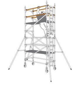
Continue the procedure until the required working height is reached, adding additional pairs of end frames, diagonal braces and fitting trapdoor platforms, as shown on previous steps. At every platform level, add horizontal braces as guardrails from the protected position within the trapdoor (as shown in Step 5).
