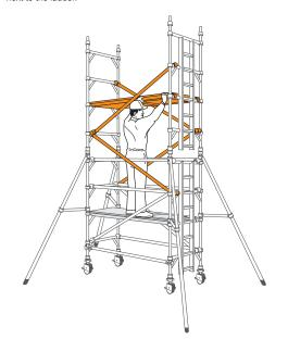
Climb up the inside of the tower and from the protected position of the trapdoor, fit guardrails to the 7th and 8th rungs (in that order) on both sides of the tower.
