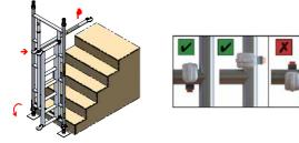
Position a second portal ladder frame higher on stairs as shown and fit other end of horizontal brace just above the bottom rung. Fit another horizontal brace as shown. This will become the higher 'upstair' end of the tower. Ensure both gates open the same direction as shown.
