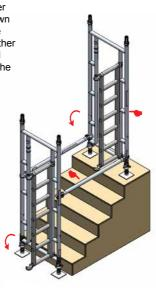
Fit two diagonal braces (blue catch) between bottom rungs of both portal ladder frames, one on each side of the tower. Claws must face downwards. The structure must be vertical to within 1cm per metre.
