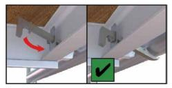
Ensure wind-locks are engaged before moving onto the deck levels.
