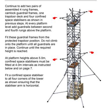
Ensure the end of the stabiliser arm contacts the wall. If it does not, adjust by unclipping and extracting the locking pin, sliding the arm until correct length and hole alignment is achieved. Reinsert the locking pin, ensuring clip is engaged. See images below:
