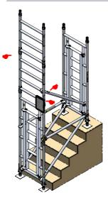
**5** Connect two 4 rung frames together and fit onto portal ladder frame as shown. Engage interlock clips. Fit one diagonal brace in position shown. Record 'Tower Designation & Safety Data' within the 'Tower Designation Information Assembly' and attach to the tower in position shown. Refer to safety data schedule for content.
