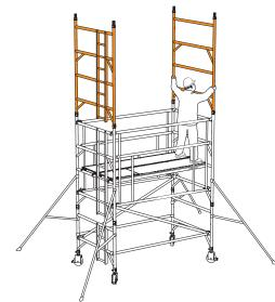
Fit two more AGRs to the end frames with the top claws on the 10th rungs, lock the AGRs in place as in Step 5. Fit a trapdoor deck on the 8th rung, with the trapdoor in line with the one below. Place a fixed deck on the 8th rung next to the trapdoor deck. The tower now has a platform height of 4.2m. If finishing at this height, move on to Step 10. If greater platform height is required, repeat Steps 7 and 8 until desired height is achieved.
