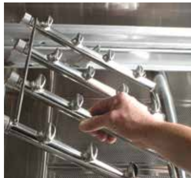
One-Piece Cast Stainless Steel Spray Assembly
