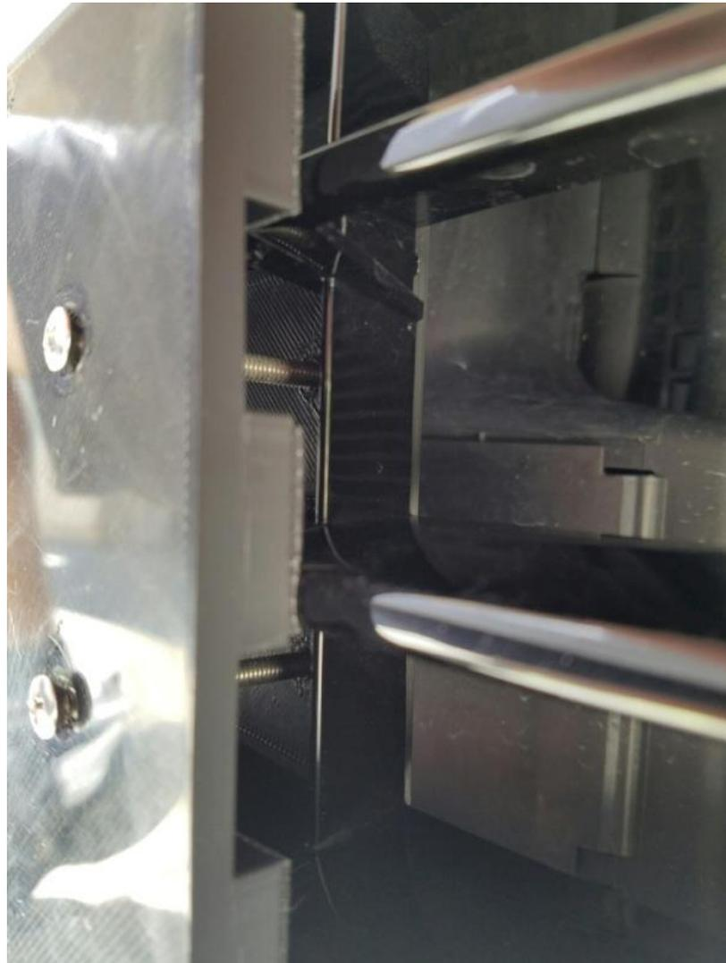
4. Install the license plate with the 4 short included screws. These are 3mm hex. There are 5 adjustment locations for the plate to dial in the location to your preference.
