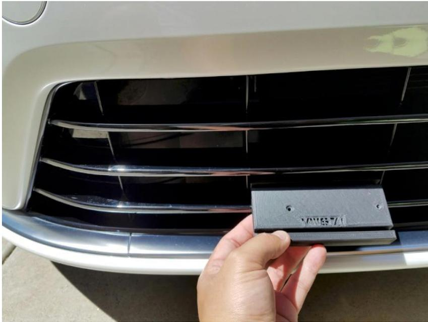
With your hand in this grill opening move the plate into position behind the grill. Warning, be very careful not to drop the back plate. Always keep a firm hold on the back plate with at least one hand.
