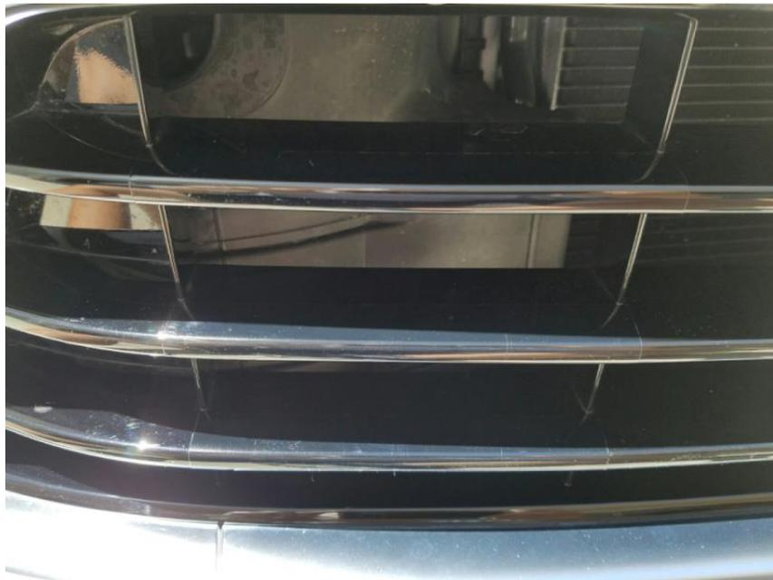
2. Install the back plate by inserting it in the grill at the location shown here, notice the orientation of the back plate indicated by the “vw671” logo.
