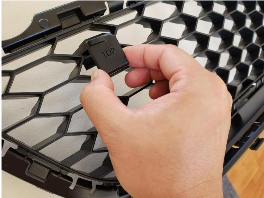
4. Once the retention bracket is sitting in the hole, rotate the bracket until it clips into place. I suggest using your thumb to push while pulling it forward with your pointer finger.
