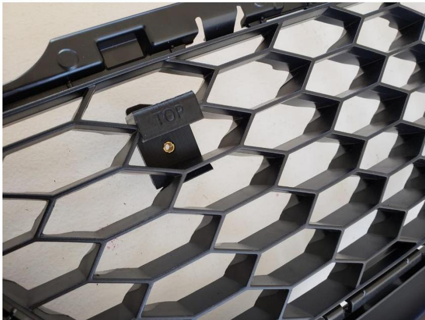
6. With all four retention clips installed it should look like this.
