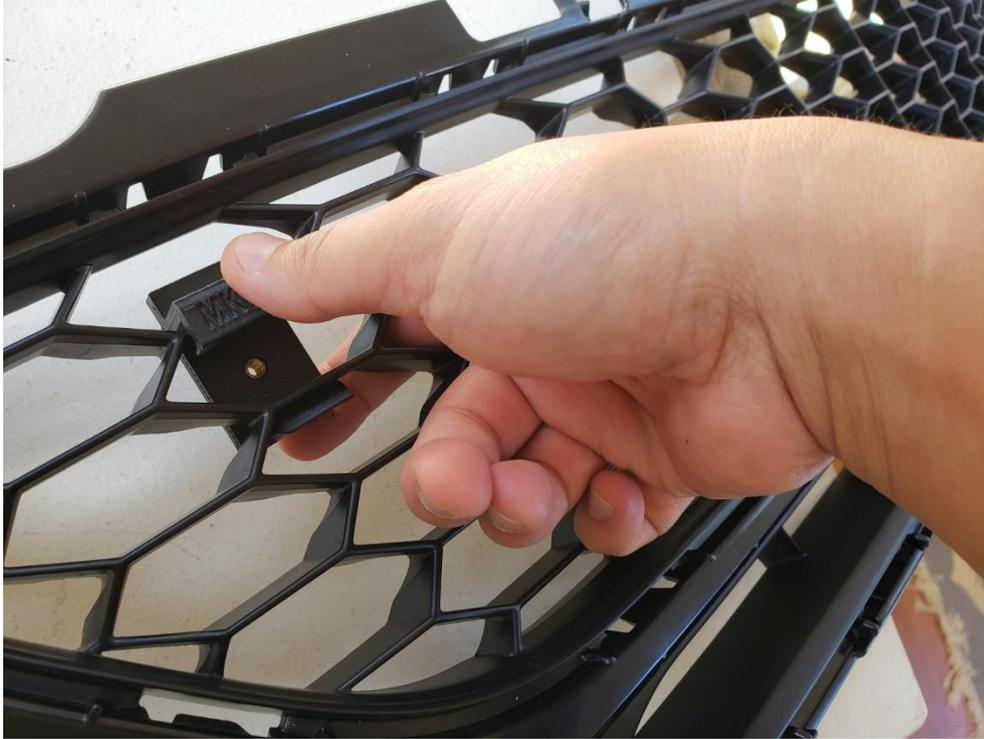
5. With all four retention clips installed it should look like this.
