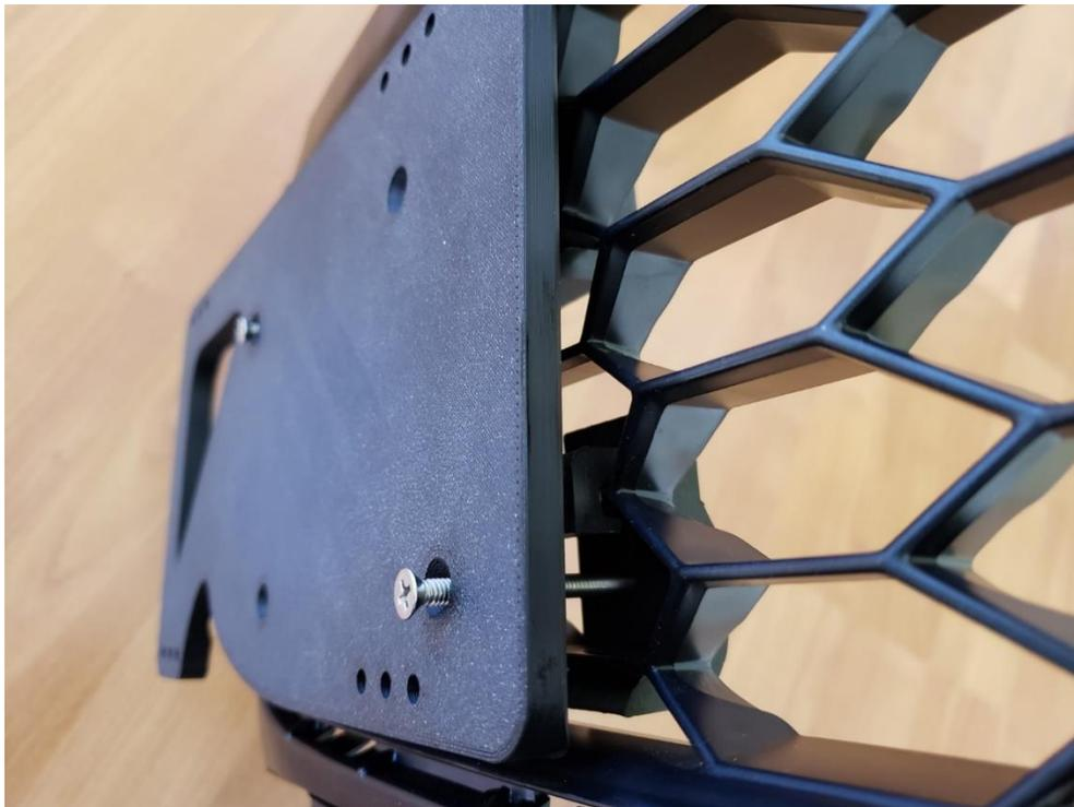
8. Now hand thread on the remaining two screws again taking care not to cross thread them. Once all 4 screws are hand threaded on use a #2 Phillips screw driver to tighten the screws. Tighten all 4 screws evenly until the main front plate sits securely on the grill and the foam padding on the back is slightly compressed. **\*Do not over tighten the screws as doing so may damage the main front plate or the grill.**
