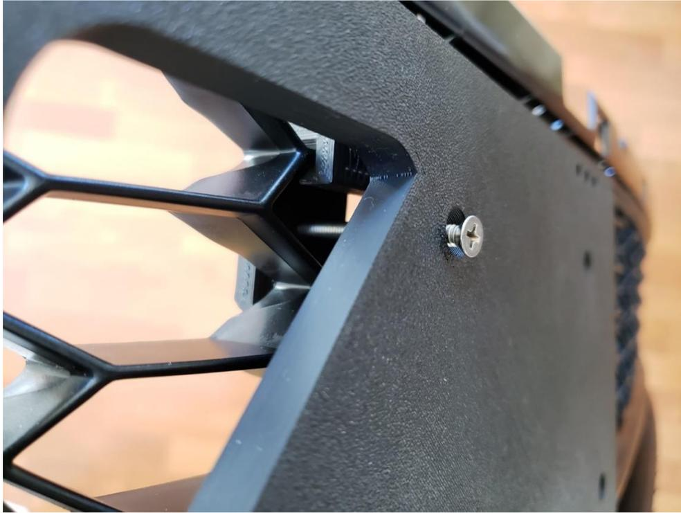
7. Next hand thread on the screw at the 4 o'clock position while viewing the alignment from the right side of the plate. Make sure that the screw is threaded on straight and not cross threaded. Do not tighten at this time.
