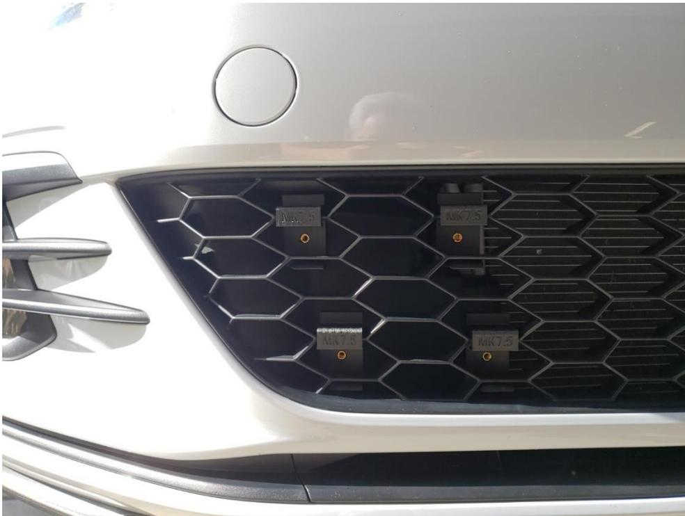
6. Position the main front plate over the retention brackets aligning the holes in the front plate with the copper screw inserts. Starting with the hole in the 10 o'clock position, hand thread one of the 8-32 x 2" flat head screw in while looking at through the cutout in the plate. Make sure that the screw is threaded on straight and not cross threaded. Do not tighten this screw at this time.
