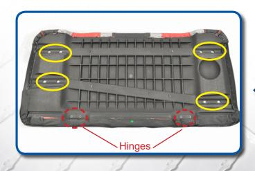
Install retained hip restraints and hinges on seat bottom of new seat. Do not overtighten.
