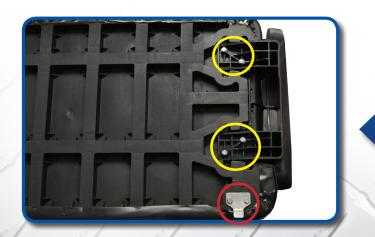
If your cart is 2012 and up install your retained hip restraints and hinges using the provided hardware then proceed to step 6.
