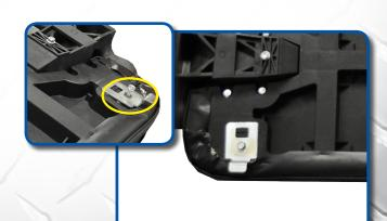
Install the lean back spacer on the base of the bracket. The longer spacer is for seat kits and the smaller one is to mount to the sweater basket. Install the M6 bolt into hexagonal shaped hole at the top of the bracket.
