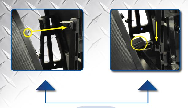
Set opening of spacer on lower mounting hook. Align upper stud with wedge and secure. Do not overtighten.
