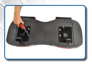
Mount the brackets to the back of your seat cushion. Do not over tighten.
