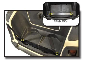
Place Seat Frame on rear of cart and secure to the Bagwell Bracket using the 10x25mm hardware from PACK 1.
