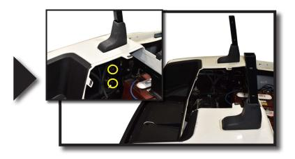
Using the factory strut bolts from STEP 1, attach the Lean Back Supports to the Main Brackets.
