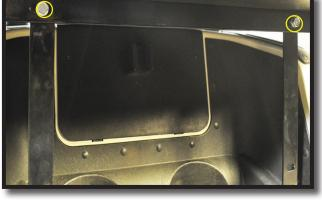
A) Attach Footrest to the Bagwell Bracket using the 10x25mm bolts from PACK 3.
