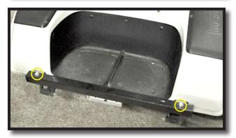
A) Install Main Seat Frame Brackets and Front Seat Lean Back Brackets to front with retained hardware.
