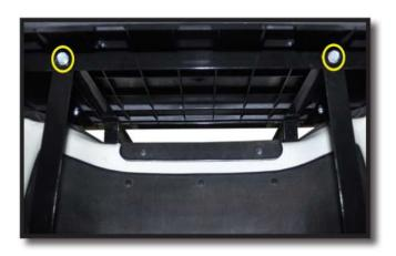
Place Seat Back Support Bar in rear of Seat Frame as shown.
