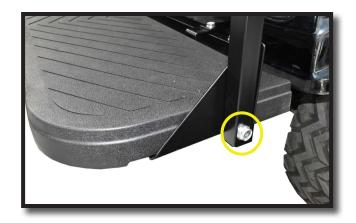
Using the 6mm hardware from PACK 4, attach the Seat Back Brackets to the Rear Lean Back Cushions as shown.
