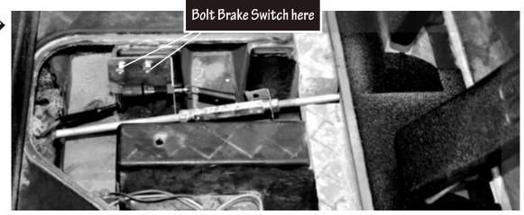
11. Plug timer relay into brake switch.
