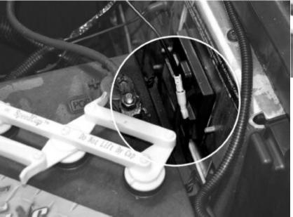
12. Connect blue wire on the new harness to the #12 wire with male connector on the #3 battery (see diagram).
