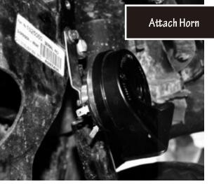
17. Attach black and orange wires on Headlight assembly to Horn.
