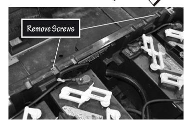
8. Using a small screwdriver, pry charge receptacle cover from vehicle.
