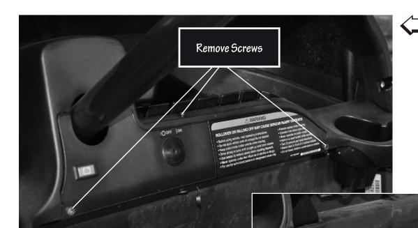
13. Remove and retain the screws that secure the dash panel to vehicle. Lift off panel.
