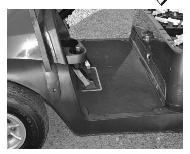
6. Remove the brake adjustment access panel.
