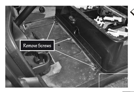
9. Remove and retain the 3 screws that secure the lower body trim to the body and lift off the lower body trim.
