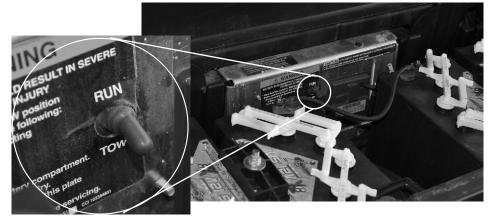
4. Disconnect the ground wire from the negative post on #4 battery on the driver side. (See Battery Diagram on the last page of these instructions)
