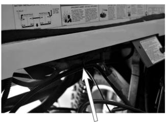
Zip tie to main harness at rear of battery compartment.
