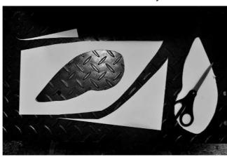
5. Align template to front cowling contour using the lower edge of the cowling as shown. Trace the inside of the cutout to mark the headlight position using a permanent marker (e.g., Sharpie<sup>®</sup>). Once you have completed the right side, flip the template over and mark the left side.
