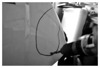
7. To cut the cowling, we recommends the use of a rotary tool (such as a Dremel <sup>®</sup> or RotoZip <sup>®</sup>) and a bit specifically made for cutting plastic.
