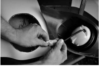
12. To fasten wiring harness to vehicle use the supplied zip ties. We recommends fastening the wiring harness to frame members in the front of the vehicle in order to prevent the harness from making contact, rubbing, or being pinched by moving parts, such as the suspension. Use two zip ties in the pedal assembly area, as shown, to tie the wiring harness to the main wiring harness. Tie the wiring harness to the main harness at the back of the battery compartment as shown.
