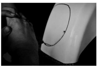
**NOTE:** To tell the left tail light assembly from the right tail light assembly, the smallest indentation in each tail light assembly surround will be towards the vehicle's CENTER.
