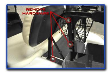
Take the seat back off the cart by removing the two back screws located on each side. Retain hardware. You will need it later.
