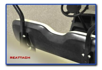
Reattach seatback using hardware from step 2.
