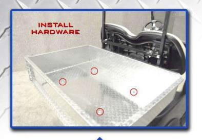
Attach cargo box to cargo box bracket using hardware from pack 4 and tighten.
