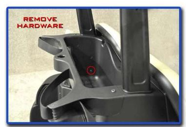
Remove upper rear canopy strut hardware. It is not necessary to remove entire canopy hardware and canopy. Retain hardware. You will need it later.
