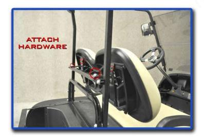
Attach seat back to seat back brackets using hardware from step 3. Attach seat back brackets to seat back bar using 45mm bolts from hardware pack 2.
