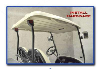
Attach the canopy by using hardware from step 2.
