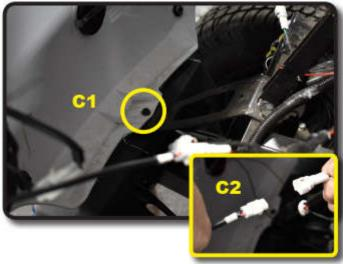
C) Remove the final 6mm screw holding the cowl on and then unplug both headlights. Keep track of all removed hardware, you will need it later.
