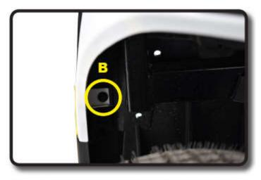
B) There is one push rivet located in each Front Fender Well which will need to be removed.
