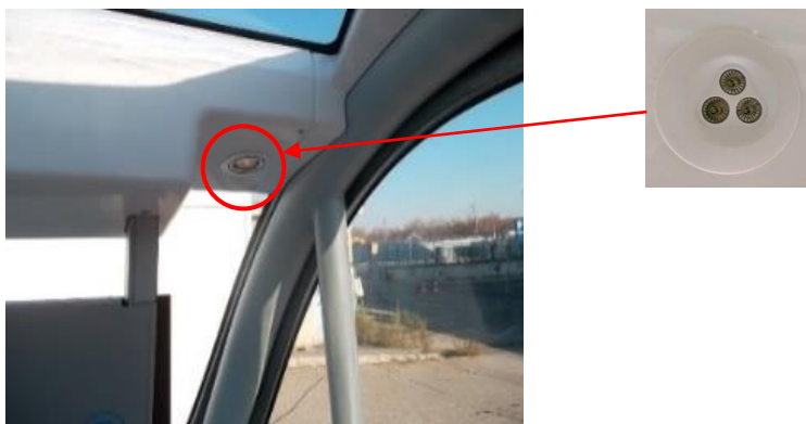
LED spots location
