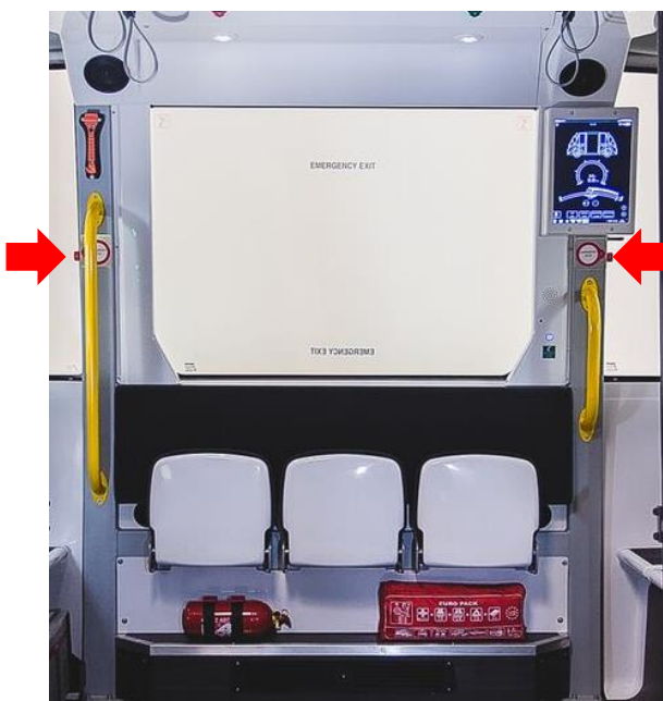
Emergency stop buttons location
