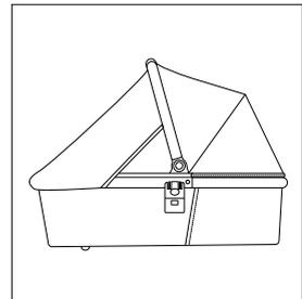
**+** **To attach:** thread the toggles to the loop fixing points on the inside of the canopy. Pull the elastic end over the foot end of the bassinet and secure the tabs on each side of the UV cover underneath the frame tube of the bassinet.
