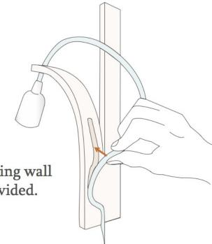
Fix bracket to wall using wall plugs and screws provided.
