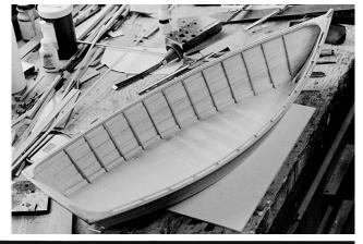
(4) Spring a batten along the top inner frame edges to check that they are all the same molded width ( $^{5}/_{64}$ " being the proper distance in from the plank) and are beveled correctly so the inwale will lie fair against them. Adjust them if necessary.
