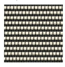
FleeceNet is a technical netweave made of polyester and polyamide with an interwoven chenille yarn. FleeceNet does not have a closed surface, making it breathable and promoting comfortable thermal conditions. The interweaving of different yarns allows for a variety of new colour combinations.
